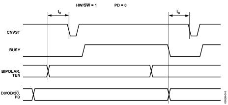
Figure 46. Hardware Configuration Timing
