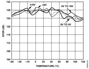
Figure 20. SFDR vs. Temperature (Excludes Harmonics)
