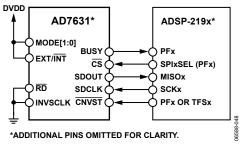
Figure 48. Interfacing the AD7631 to SPI Interface
