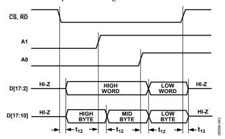
Figure 40. 8-Bit and 16-Bit Parallel Interface
