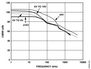
Figure 29. Analog Input CMRR vs. Frequency
