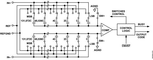
Figure 25. ADC Simplified Schematic
