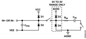
Figure 28. Simplified Analog Input
