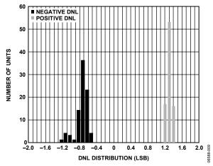
Figure 9. Differential Nonlinearity Distribution, Bipolar 5 V Range (86 Devices)
