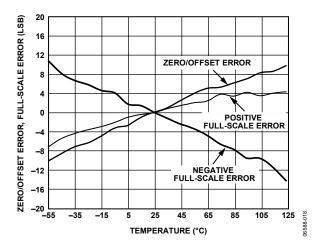
Figure 18. Zero/Offset Error, Positive and Negative Full-Scale Error vs. Temperature, All Normalized to 25℃
