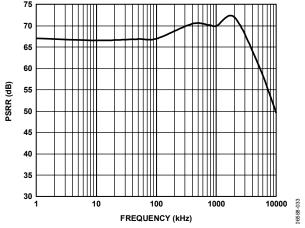
Figure 33. AVDD PSRR vs. Frequency
