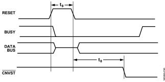
Figure 36. RESET Timing
