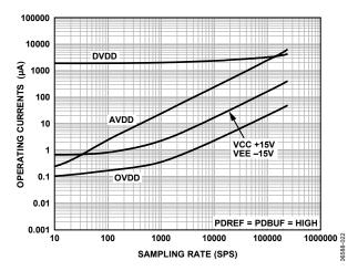
Figure 22. Operating Currents vs. Sample Rate
