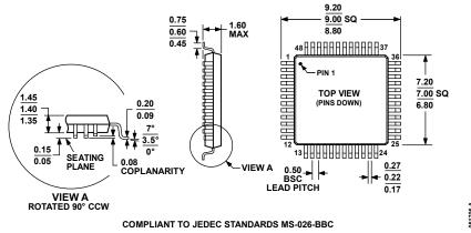
Figure 49. 48-Lead Low Profile Quad Flat Package [LQFP] (ST-48) Dimensions shown in millimeters
