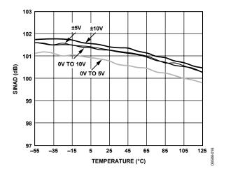
Figure 16. SINAD vs. Temperature
