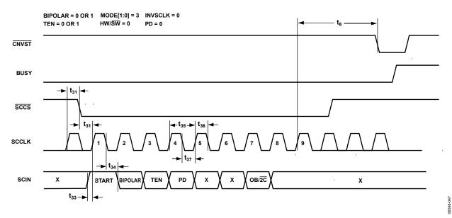
Figure 47. Serial Configuration Port Timing
