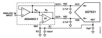
Figure 31. Single-to-Differential Driver Using the ADA4922-1
