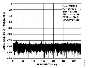
Figure 11. FFT 20 kHz, Bipolar 5 V Range, Internal Reference
