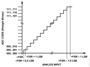
Figure 26. ADC Ideal Transfer Function
