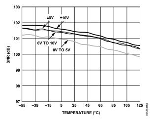
Figure 13. SNR vs. Temperature
