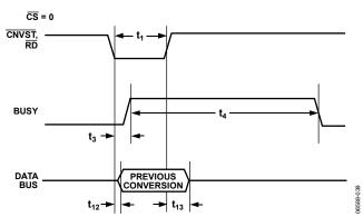
Figure 39. Slave Parallel Data Timing for Reading (Read During Convert)
