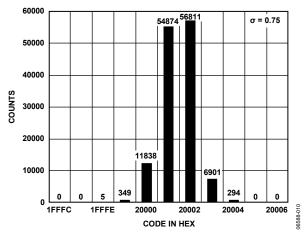
Figure 10. Histogram of 261,120 Conversions of a DC Input at the Code Transition, Bipolar 5 V Range
