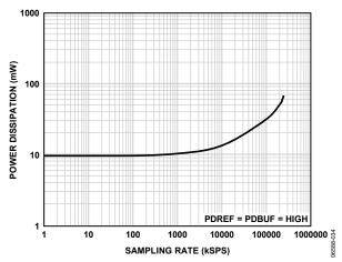
Figure 34. Power Dissipation vs. Sample Rate
