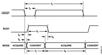
Figure 35. Basic Conversion Timing
