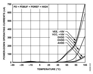
Figure 23. Power-Down Operating Currents vs. Temperature
