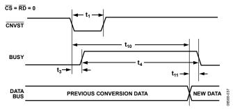
Figure 37. Master Parallel Data Timing for Reading (Continuous Read)
